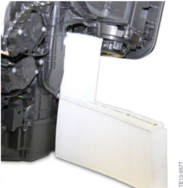
Heating and air-conditioning unit with microfilter pulled out
